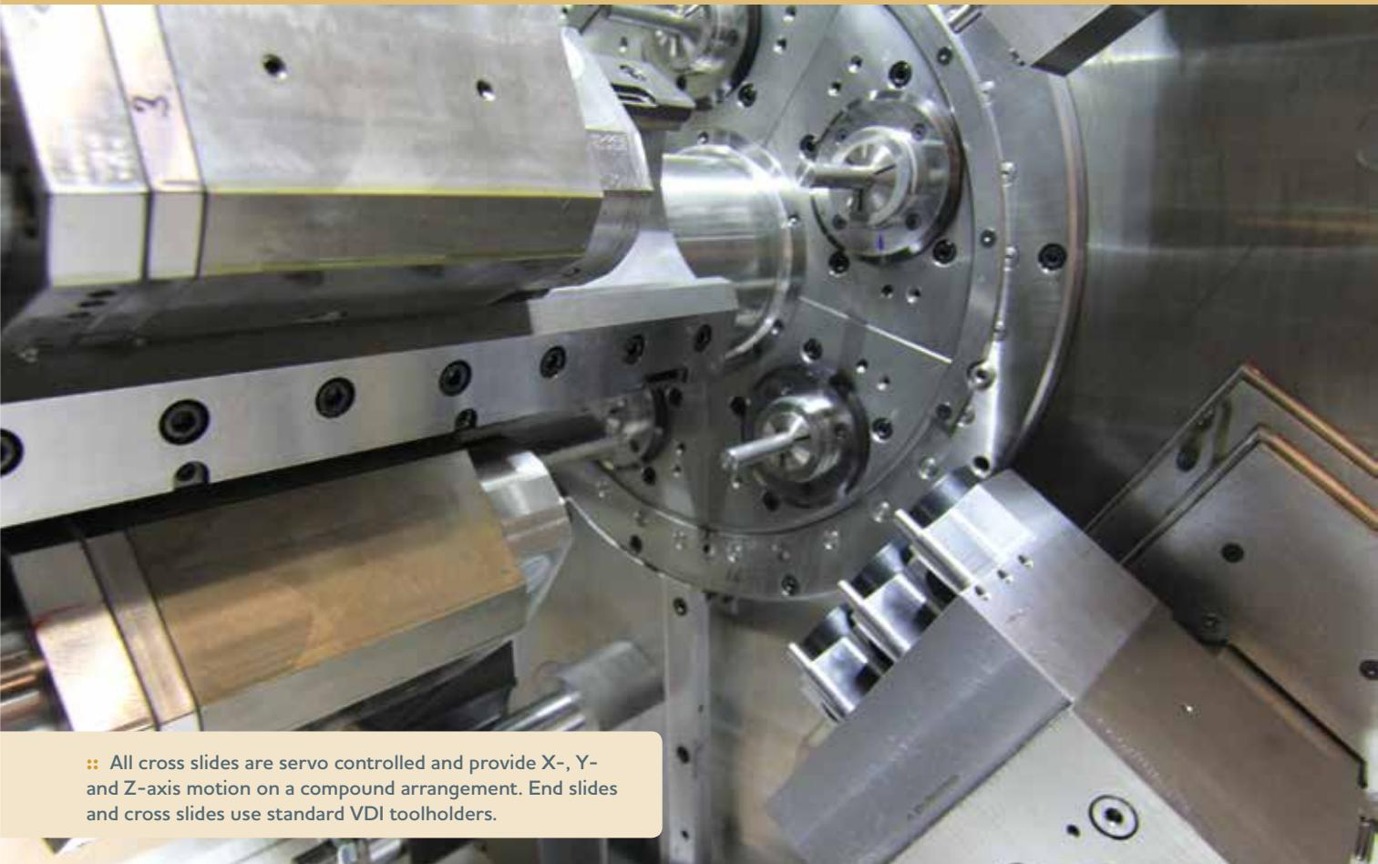
⚙️ All cross slides are servo controlled and provide X-, Y- and Z-axis motion on a compound arrangement. End slides and cross slides use standard VDI toolholders.
